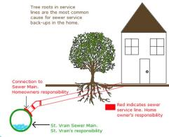
If you have ever had a slow or stopped up drain line and suspect roots, St. Vrain Sanitation District recommends cutting the roots, and then applying a product called Root-X. This product is designed to remove the roots from your sewer service line for up to 12 months without harming trees or shrubs. It won't fix your service line but may prolong its life and prevent costly backups and line cleaning bills.
